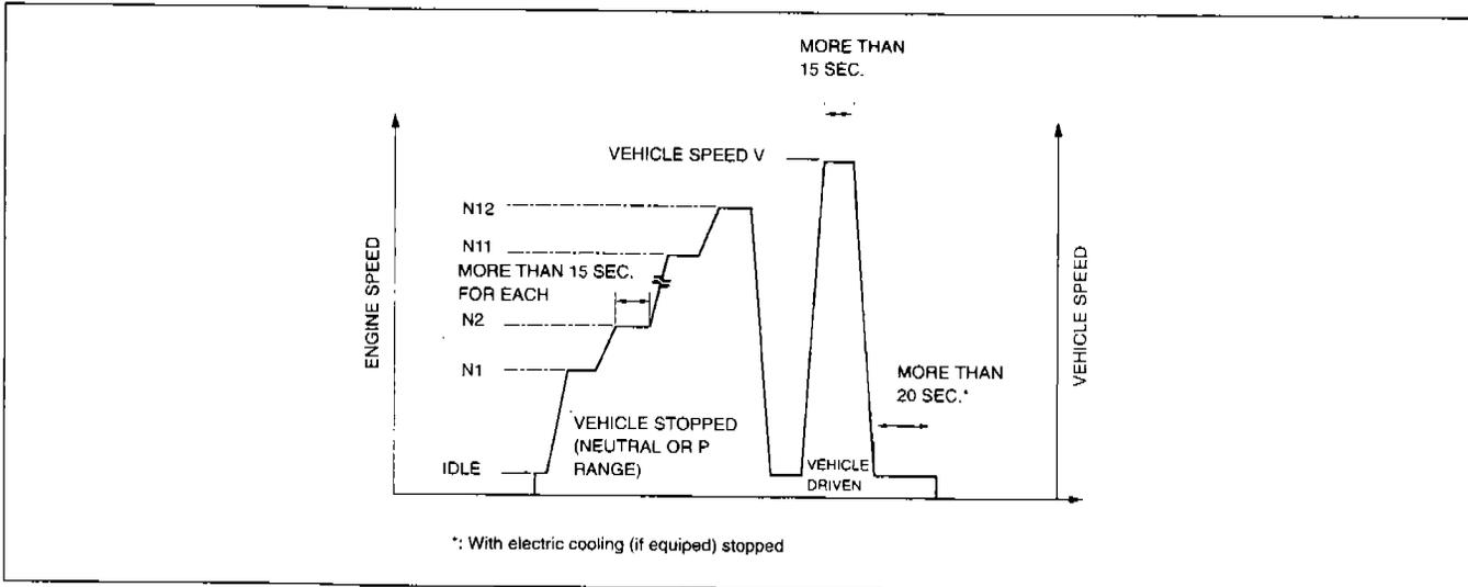
MODE 1-A Engine speed and vehicle speed table
