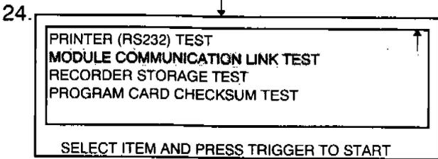
Select "MODULE COMMUNICATION LINK" and press "TRIGGER"
