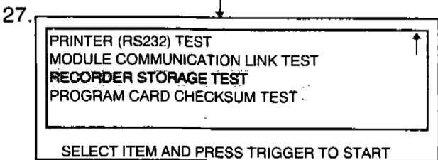
Select "RECORDER STORAGE TEST" and press "TRIGGER"
