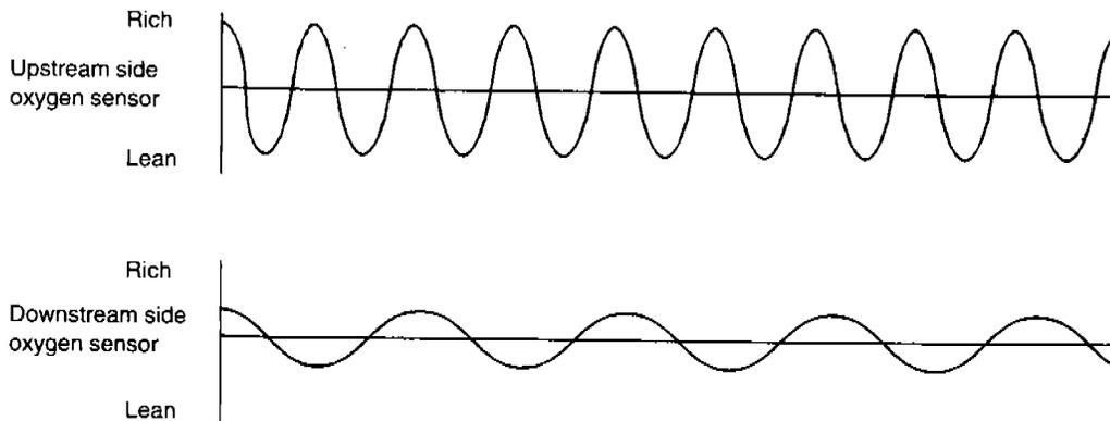
Fig.11 Catalytic converter deteriorates
