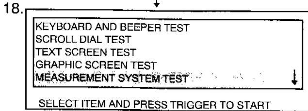
Select "MEASUREMENT SYSTEM TEST" and press "TRIGGER".
