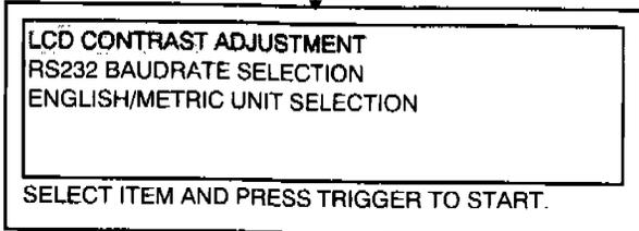
Select "**LCD CONTRAST ADJUSTMENT**" and press "**TRIGGER.**"
