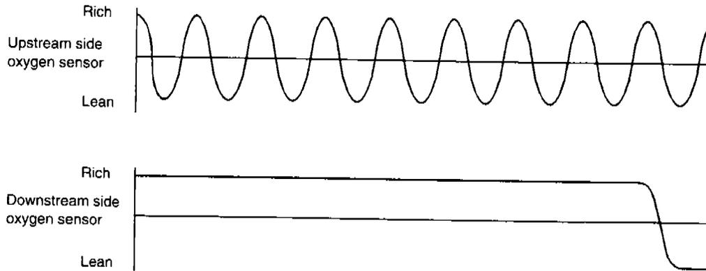
Fig.3 Catalytic converter deteriorates
