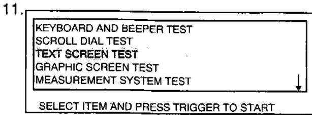
The **TEXT SCREEN TEST** checks the letter display condition.
