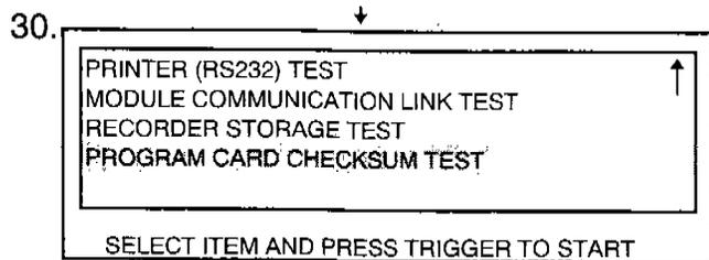
The **PROGRAM CARD CHECKSUM TEST** checks the program card condition.
