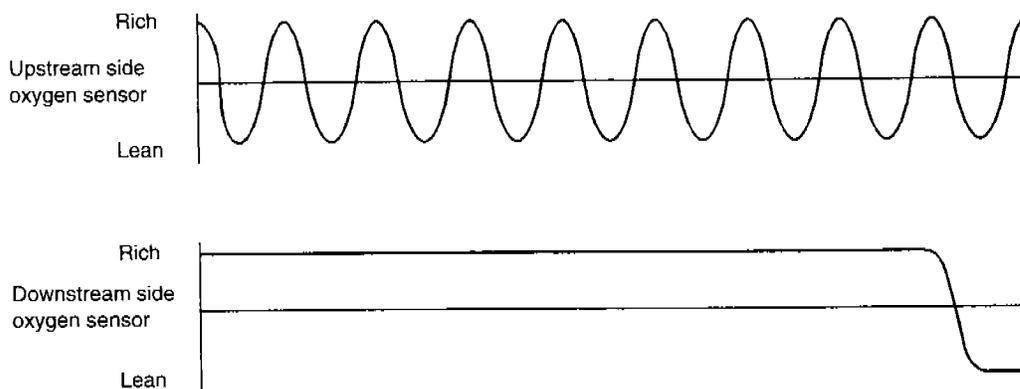
Fig.5 Catalytic converter deteriorates
