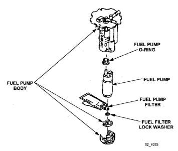
**NOTE:** Warranty claims submitted for a Fuel Pump Assembly <u>will be denied or subject to debit</u> when an individual replacement part could have been used to repair the vehicle (i.e. Fuel Pump Body, Fuel Pump, Fuel Pump Filter, etc.).
